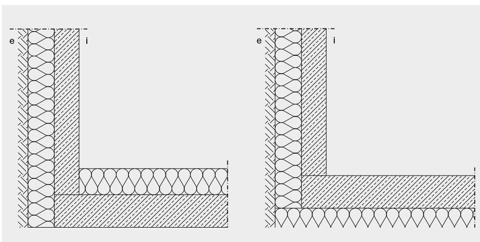
Image 4.7 Depiction of an “insulation gap” (left) and the optimized junction (right)
