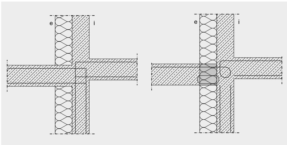
Image 4.6 Depiction of a penetration of the insulation layer without decoupling (left) and the optimised thermally separated connection (right)
