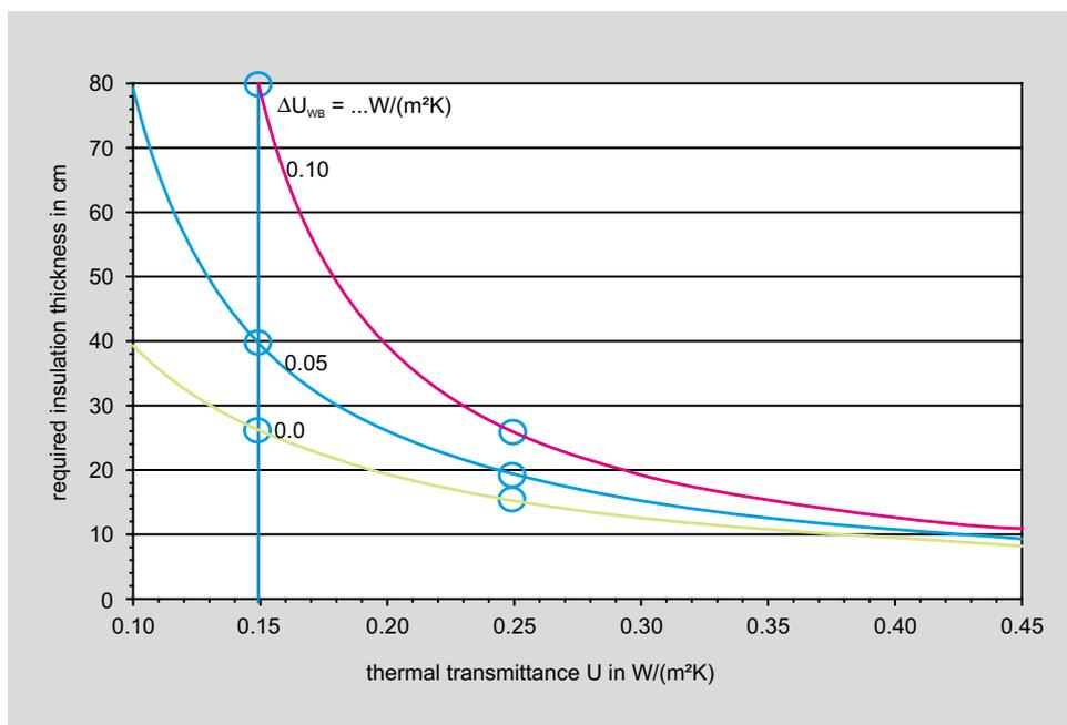
Image 4.3 Influence on the required insulation thickness by the thermal bridge surcharge  $\Delta U_{WB}$
