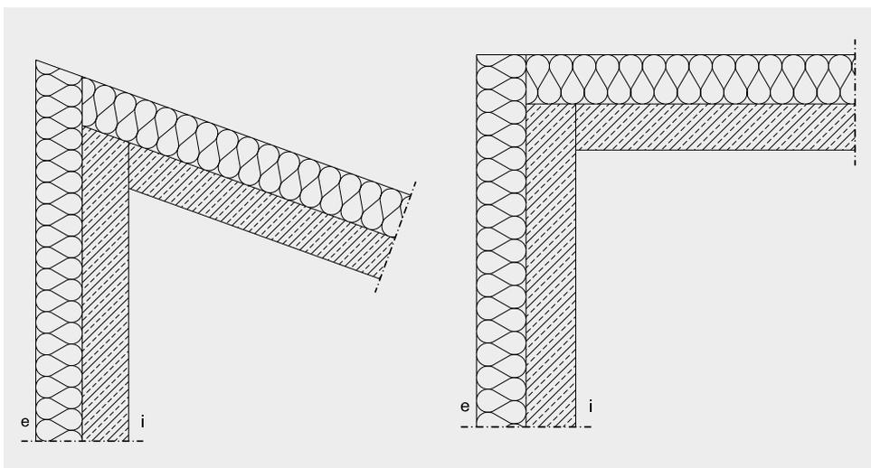
Image 4.5 Depiction of a sharp outside corner (left) and an optimized design (right)
